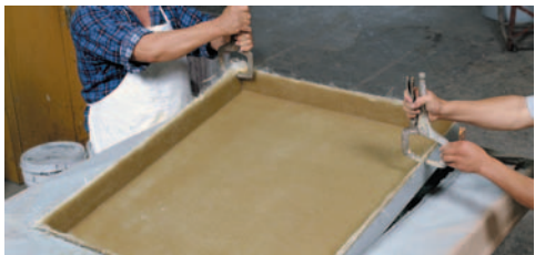
7. Once the resin cures and hardens, the parts are removed from the mold.
