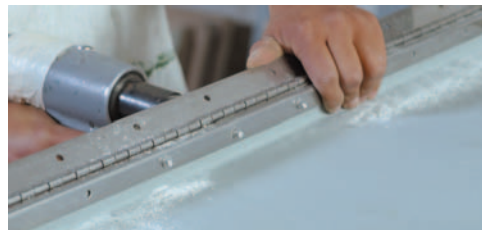
8. The door is installed to the enclosure base using a heavy duty, continuous stainless steel hinge.
