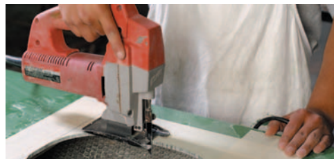
10. An opening is cut into a door for an optional gasketed window. Holes and cutouts can be provided to customer specifications.
