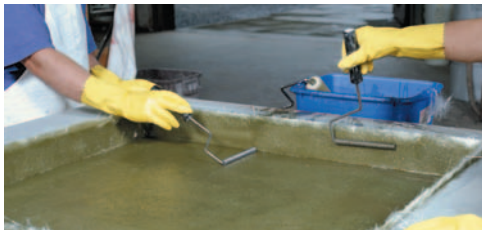
5. A roller is used to push out entrapped air and compress the laminate before the next layer is added.
