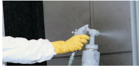
2. The outer surface of the enclosure is sprayed into the enclosure mold using a marine grade gelcoat.
