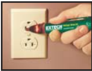
Line outlet testing
