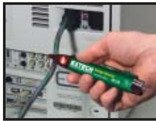
Locate power cord breaks
