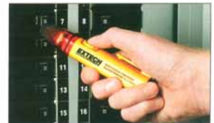
Non-contact AC Current measurements from 200mA to 1000A
