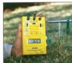
Check resistance between earth and grounding rod.
